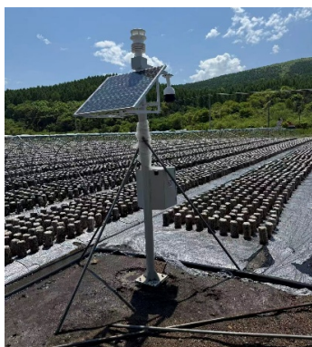
Figure 15 GIES ground station (Photo taken by WANG Yichun on May 24, 2025)
