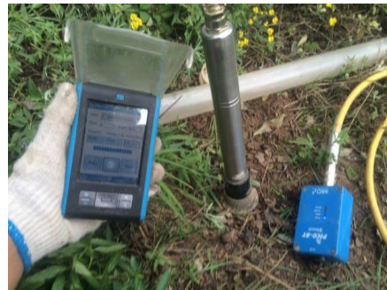
Figure 4 Soil water content measured by TDR
